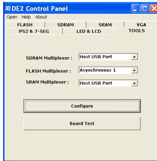
Figure 3.8. TOOLS window of the DE2 Control Panel.
