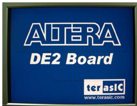
Figure 2.3. The default VGA output pattern.
